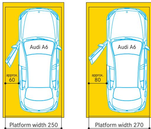
Depending on the vehicle model and the parking position of the vehicle on the platform, the space for opening the door varies. For comfortable conditions for getting in and out of the car, we recommend platform widths of 270 cm.
