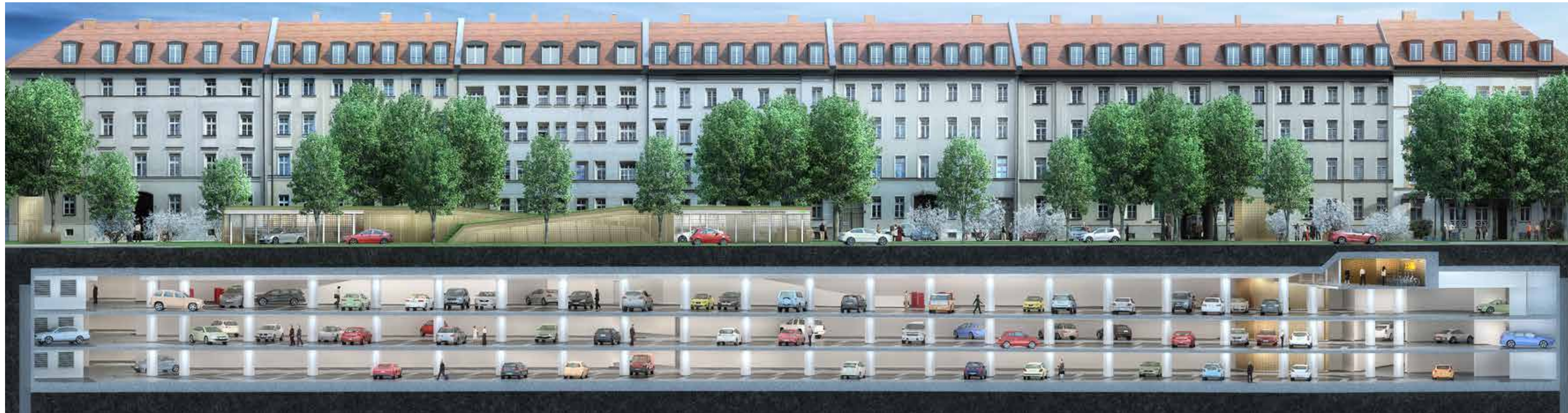
Current project: the underground car park beneath Thomas-Wimmer-Ring is part of the 'TOM and HILDE' project duo. These state-of-the-art, incredibly convenient parking spaces extend 140 metres long and 30 metres deep. Graphics: WÖHR + BAUER GmbH
